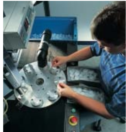
This state-of-the-art unit connects plastic parts by means of ultrasonic welding.
